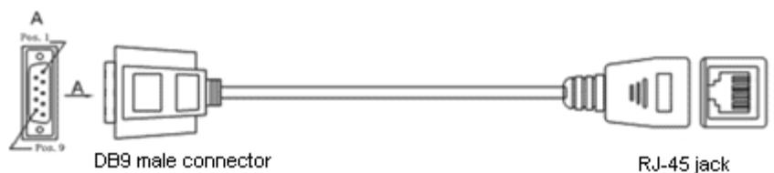
Figure 1-26: Balanced cable with the RJ-45 jack
