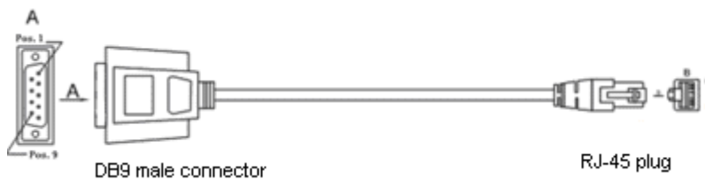
Figure 1-25: Balanced cable with the RJ-45 Plug
