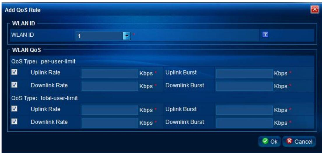
Note: On Ruijie AC device, QoS rate limit is based on 8 kbps. On RUIL, QoS rate limit is based on kbps. Therefore, user configuration data may be different from the actual configuration on the device. For example, the rate configured by the user is 65 kbps, but the actual rate on the device is 64 kbps. The rate displayed by RUIL to users is also 64 kbps.
