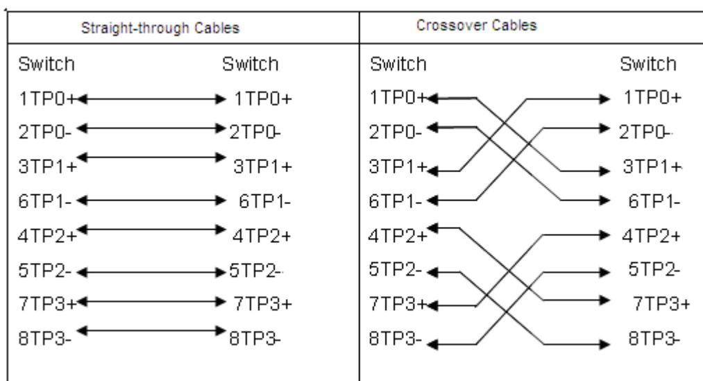
In addition to the above cables, the 100BASE-TX/10BASE-T can also use 100-ohm Category-3, 4, 5 cables for 10 Mbps, and 100-ohm Category-5 cables for 100 Mbps, both of which can be up to 100 m. Figure A-2 shows the pinouts of the 100BASE-TX/10BASE-T.
