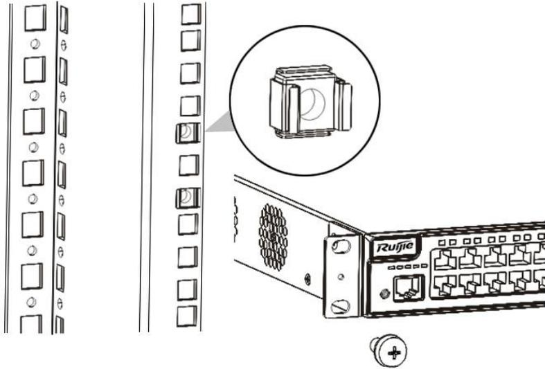
Use the supplied M6 screws and cage nuts to securely attach the mounting brackets to the rack, as shown in Figure 3-3.
