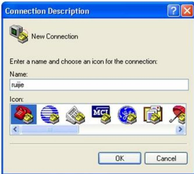
3) Enter the name of the new connection and click **OK**, the interface as shown in figure 4-3 is displayed. Choose the serial port used currently in the column [use when connecting].
