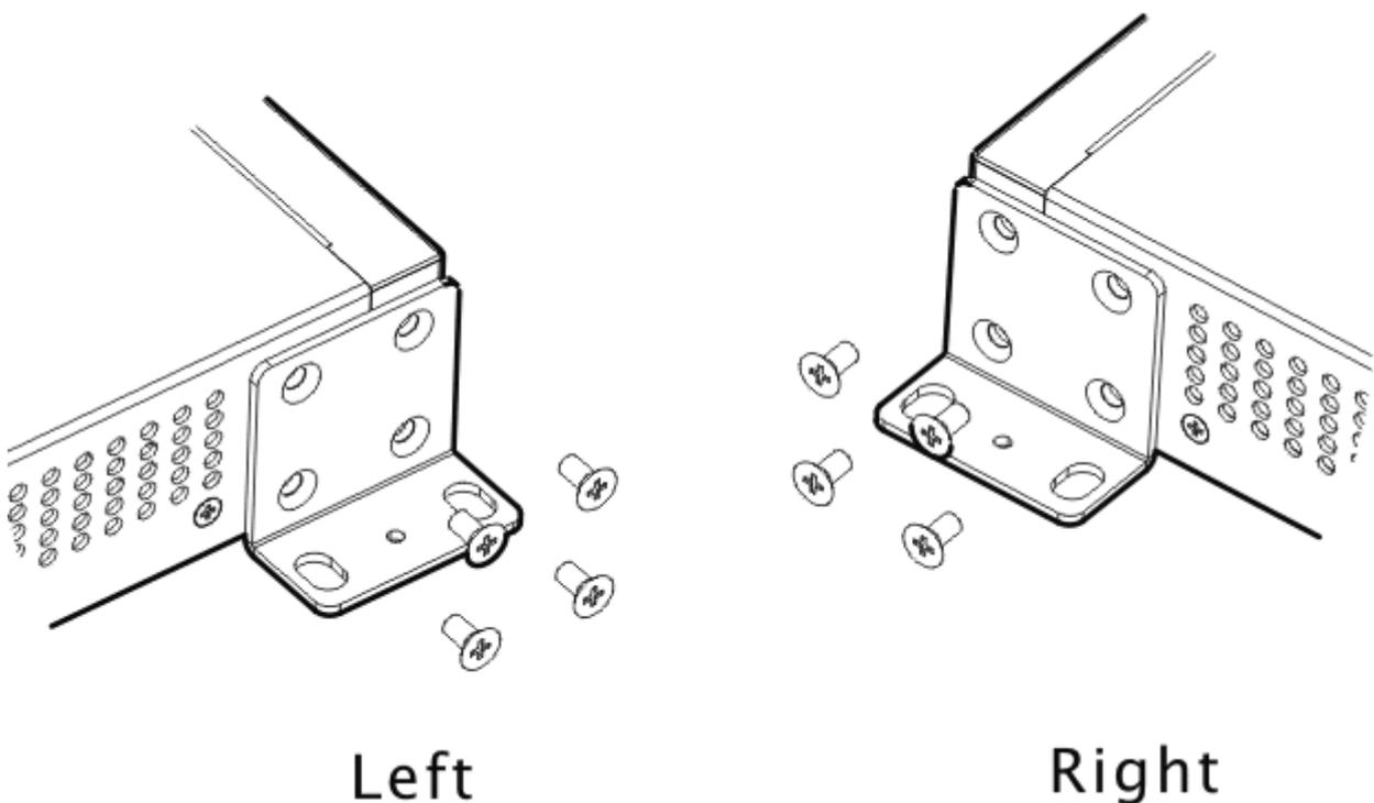
Align the mounting holes in the mounting bracket with the mounting holes in the rack, as shown in Figure 3-2.
