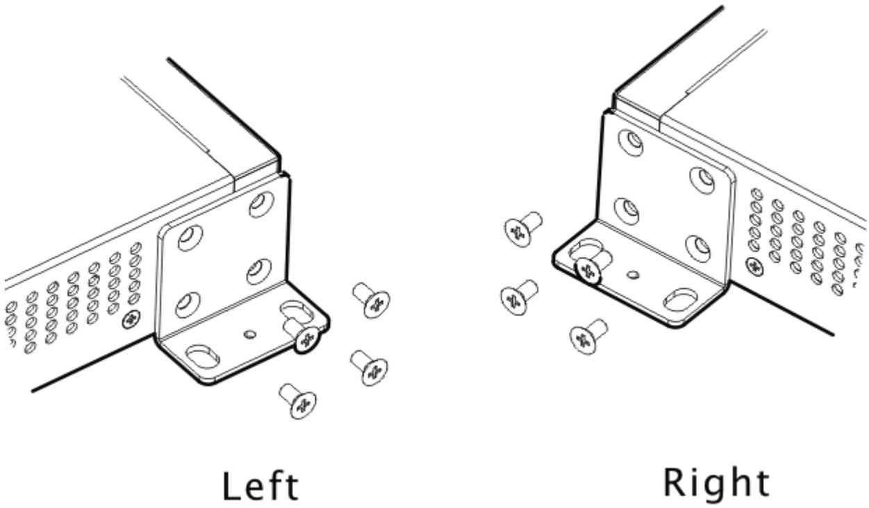
Use the expansion screws to securely attach the mounting brackets on the wall, as shown in Figure 3-5.
