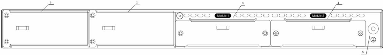
Note: 1. Slot for the power supply module 1    4. Slot for the extension module 2
