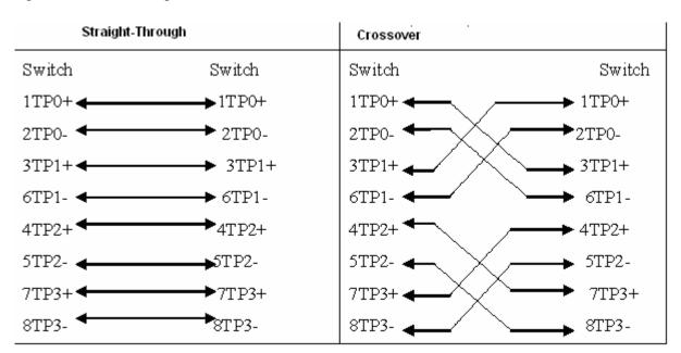
Figure A-1 Schematic Diagram for the Four Twisted Pairs of the 1000BASE-T
